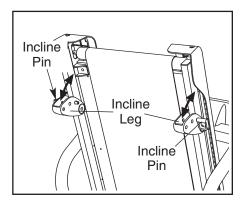
the other incline leg in the same way. CAUTION: Before using the treadmill, make sure that both incline legs are at the same height and that both incline pins are fully inserted into the incline legs.
